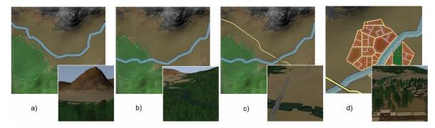
**Figure 2:** A procedural sketching session and resulting 3D virtual world (insets): a) natural environment mountains, river and forest. b) the river is rerouted to run through the forest. c) a road is placed across the river. d) city created along the river banks.
