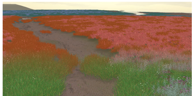
Figure 5: The seamless transition between the different LODs. Far-away LOD is colored blue. Billboards are colored red, and the plant models have their regular color.
