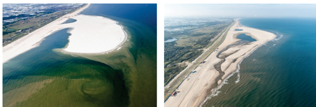
Figure 2: An example of a ‘Building with Nature’ project [de Vriend et al. 2014]. On the left image, a lot of sand is placed, which is transformed by ecological processes in the area shown in the image on the right.
