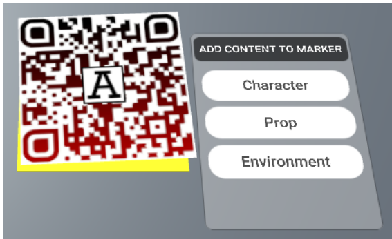
Figure 4: Marker programming space with marker placed on top of it. The menu appeared next to the marker to add content to it.
